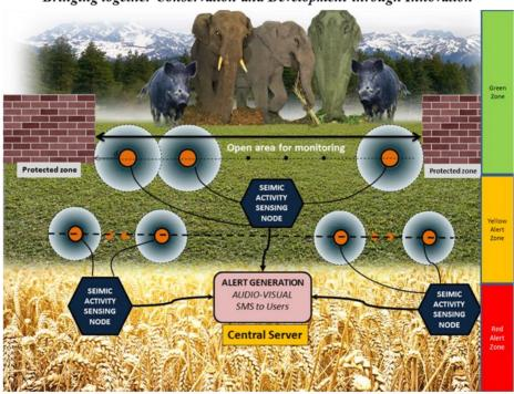
AI based Seismic Sensing is an innovative comprehensive technological solution, from CSIR-CSIO, Chandigarh, for early detection of crop raiding animals and subsequent alert generation to the concern users and farmers to avoid human-wildlife conflict.
