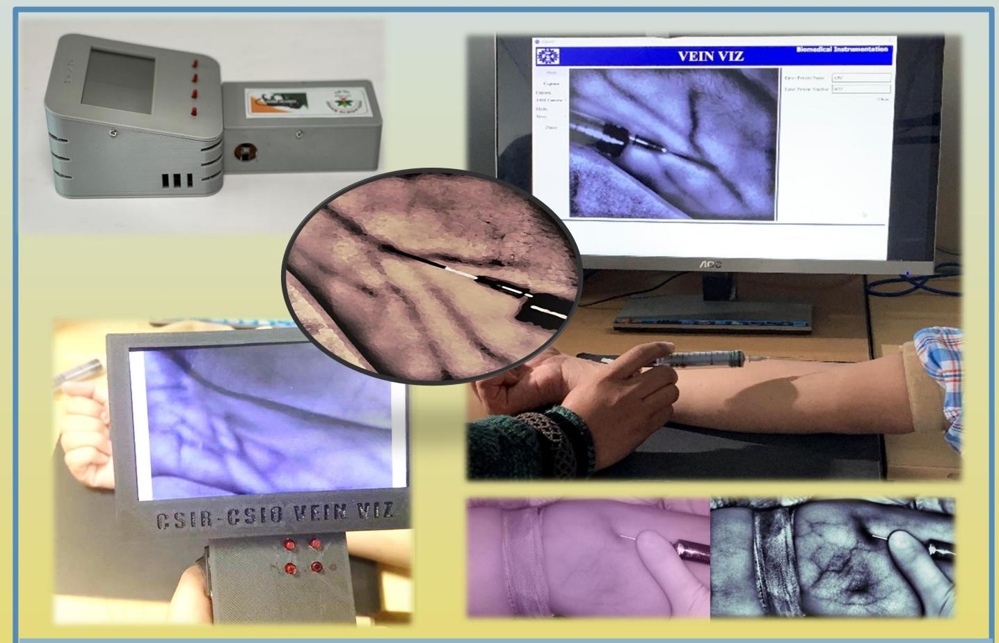
Real-time vein detection, localization and visualization device based upon near infrared light and digital imaging. It is useful towards finding and visualizing clinically relevant difficult to access veins in children, obese and elderly. This device could assist Phlebotomists and healthcare workers improve patient experience by reducing number of sticks, lower catheter dwell time, and precise venipuncture avoiding associated complications.
